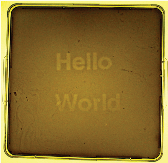
Figure TF31-2: By introducing new genes into E. coli , the bacteria were made sensitive to light. In this example, by a team from the University of Texas at Austin and the University of California, San Francisco, a thin film of bacteria was grown in a Petri dish and exposed to patterns of light with the message “Hello World.” Each bacterium in the film responded by changing color depending on the light level it was exposed to.
