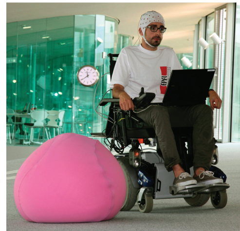
Figure TF32-1: A variety of existing, functional prosthetics. (a) The “Luke arm” built by DEKA Corp.; (b) an exoskeleton built at the Kazerooni Lab, University of California, Berkeley; (c) an EEG-controlled wheelchair, developed by José del R. Millán’s group at the École Polytechnique Fédérale de Lausanne (EPFL, Switzerland).
