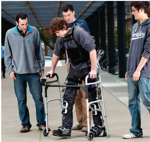
Figure TF32-1: A variety of existing, functional prosthetics. (a) The “Luke arm” built by DEKA Corp.; (b) an exoskeleton built at the Kazerooni Lab, University of California, Berkeley; (c) an EEG-controlled wheelchair, developed by José del R. Millán’s group at the École Polytechnique Fédérale de Lausanne (EPFL, Switzerland).
