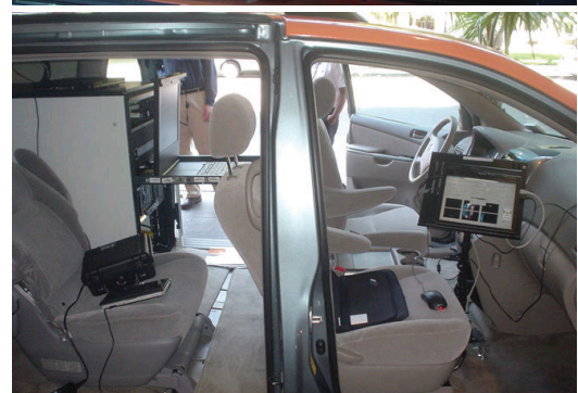
Figure TF29-3: A TeleAtlas van showing the imaging and laser equipment and the computation hardware inside the van.
