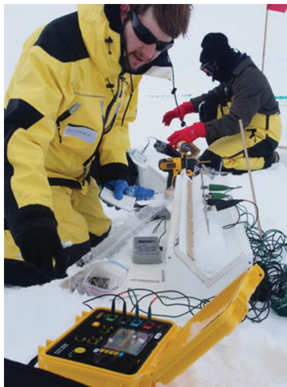
Figure TF6-5: University of Utah mathematics Ph.D. student Christian Sampson measures the electrical conductivity of a sea-ice core during the Sea Ice Physics and Ecosystem eXperiment in 2012. Electrical clamps are attached to nails inserted along the length of the ice core. (© Wendy Pyper/Australian Antarctic Division.)
